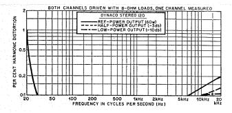
At 1,000 Hz, harmonic distortion was under 0.1 per cent from 0.1 watt to 70 watts. Intermodulation distortion was under 0.1 per cent below 1 watt and reached 0.2 per cent at 60 watts. The frequency response was perfectly flat, as indicated by our meters, from 20 to 20,000 Hz. Hum and noise with an open input were 80 db below 10 watts, or 88 db below 60 watts. An input signal of 0.7 volt will drive the Stereo 120 to 10 watts per channel, more than enough for any normal listening situation.
