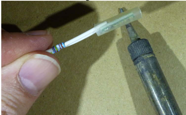
Figure 9-Shrink the tubing by rubbing the tip of the iron along the tubing on all sides
