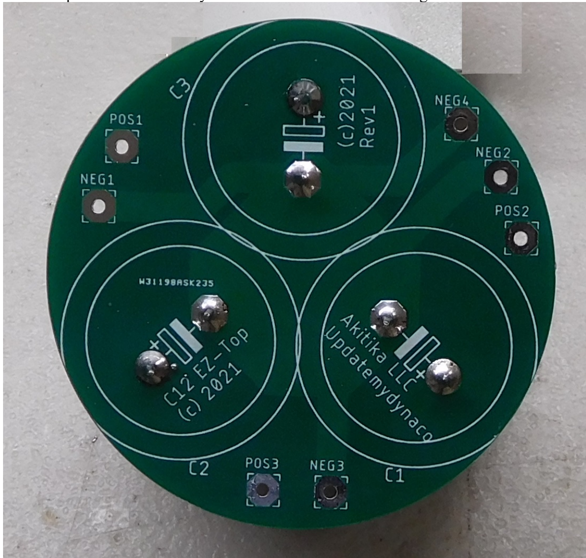
Figure 3-3 30 mm diameter capacitors take the space of one 2.5" diameter capacitor
