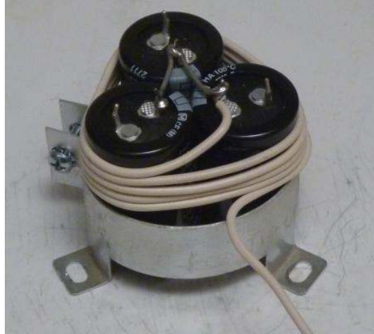
Figure 6-Inductor wound around the new C7
