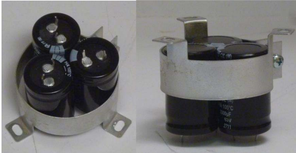
Figure 3-3 25 mm diameter capacitors take the space of one 2" diameter capacitor
