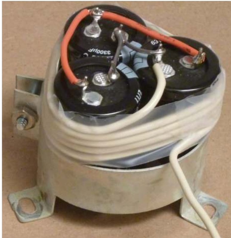
Figure 7-Adding red wires to connect positive terminals
