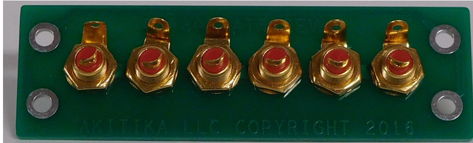
Figure 2-One of 4 jack-fields, before addition of ground wires
