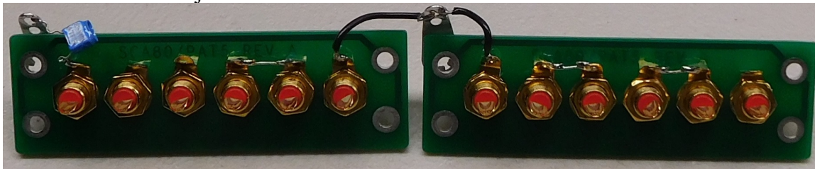
Figure 3-Right Channel Jacks with grounds and 0.01 uF cap
