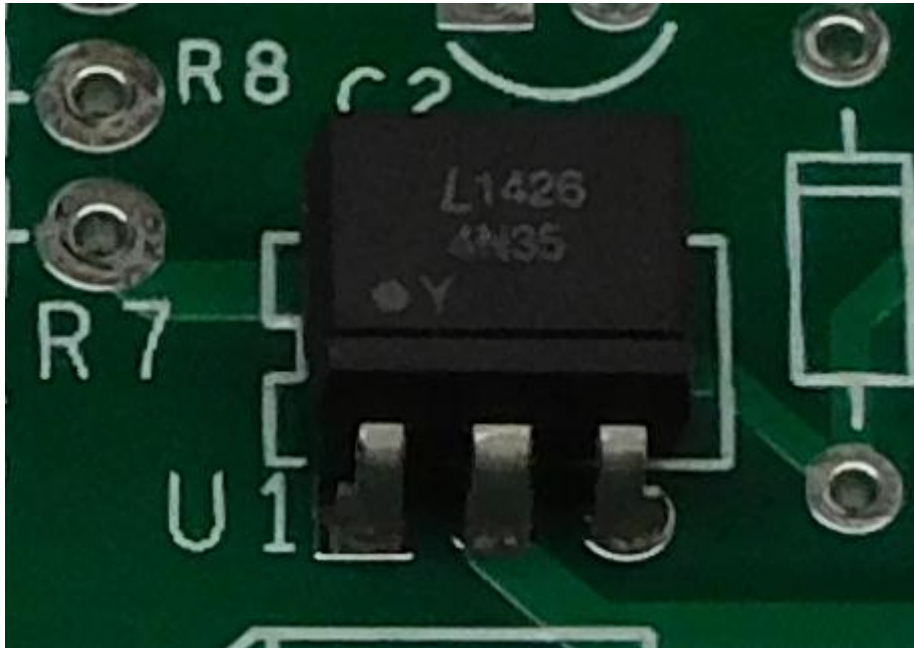
Figure 3-Pin 1 of the opto-isolator is indicated by the dot and the ridge in the package
