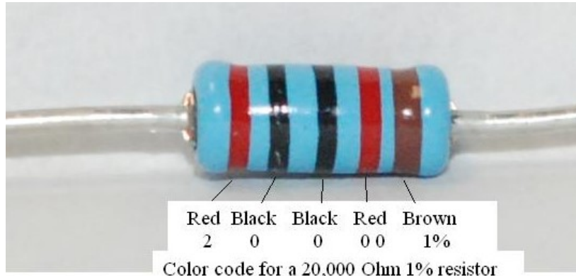
Figure 11-demonstrating the resistor color code
