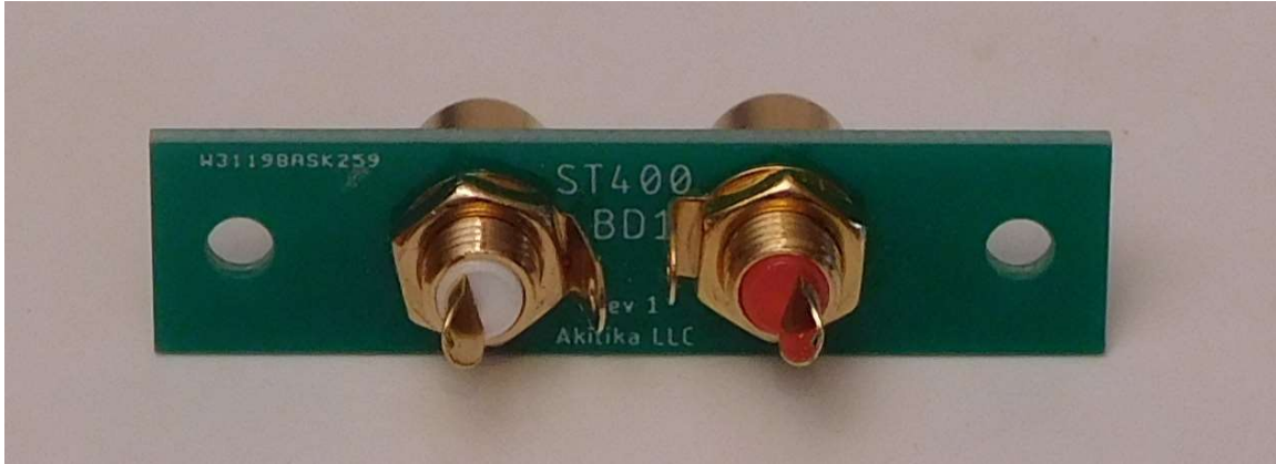
Figure 4-Mount the RCA jacks as shown onto the PCB
