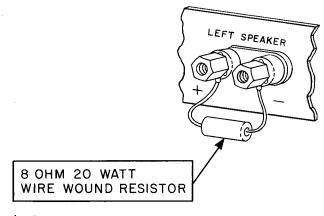
(RESISTOR CAN ALSO BE 16 OHM 20 WATT OR 4 OHM 20 WATT WIRE WOUND)
