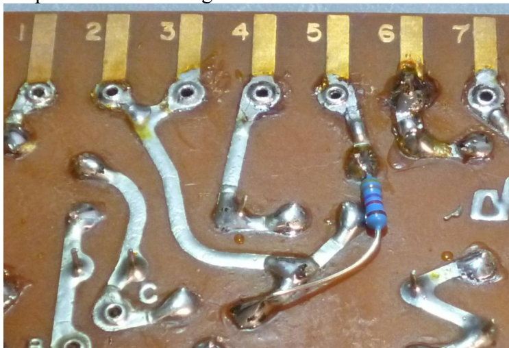
Figure 6-Final step of R30 installation in those cases where holes don't already exist on the PCB
