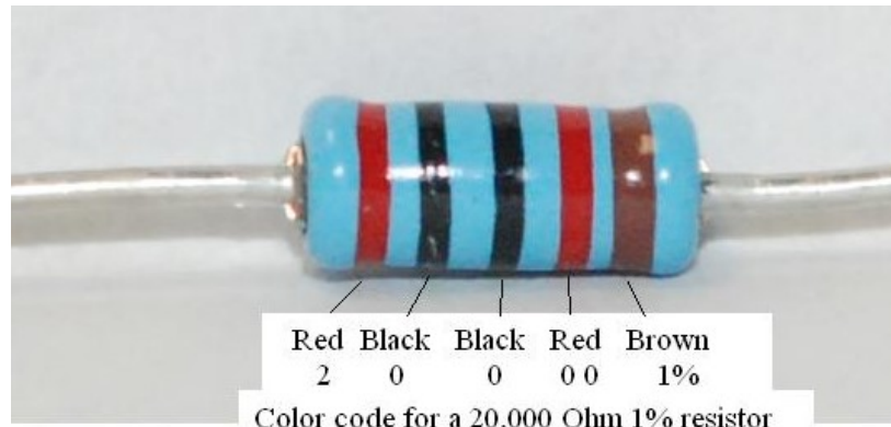
Figure 7-demonstrating the resistor color code
