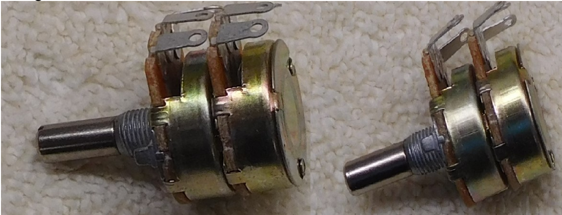
Figure 4- gently bend the leads away from the body (before on left, after on right)
