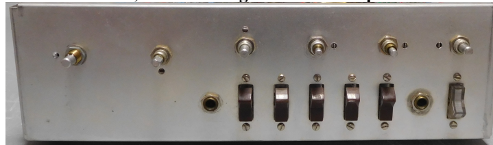
Figure 3-Viewing the structural front panel with the cosmetic front panel removed
