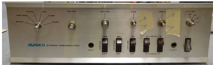
Figure 2-knobs removed, note markings for clockwise positions of tone controls
