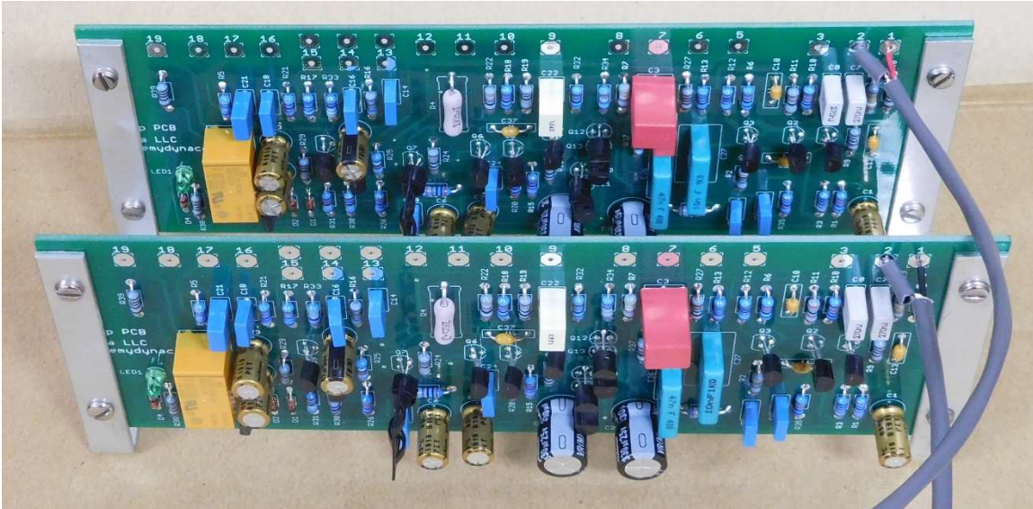
Figure 10-Re-use the original 4-40 screws to re-attach mounting brackets to the PCBs
