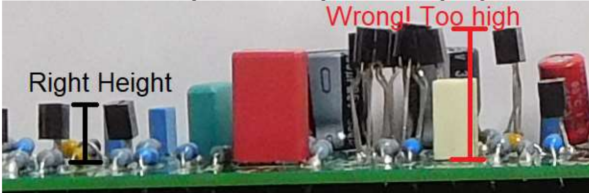
Figure 3-Proper height for transistor installation
