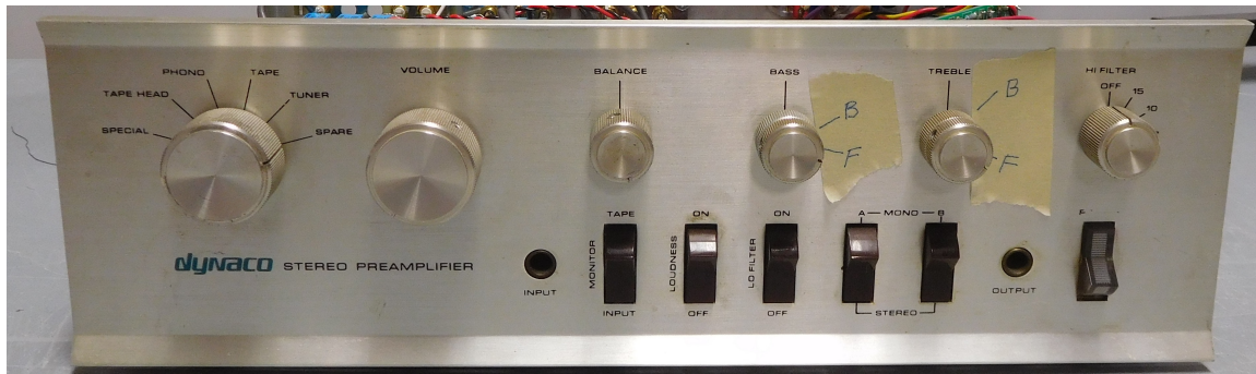
Figure 1-Mark the fully clockwise positions of the front and back tone control knobs
