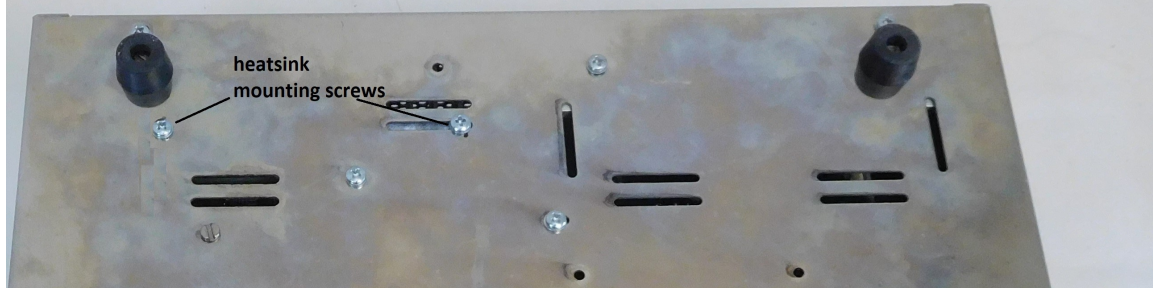
Figure 7-use 6-32x3/8" screws to mount the heatsink
