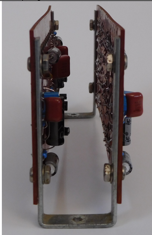
Figure 1-Both PCBs reassembled onto U brackets, ready for installation
