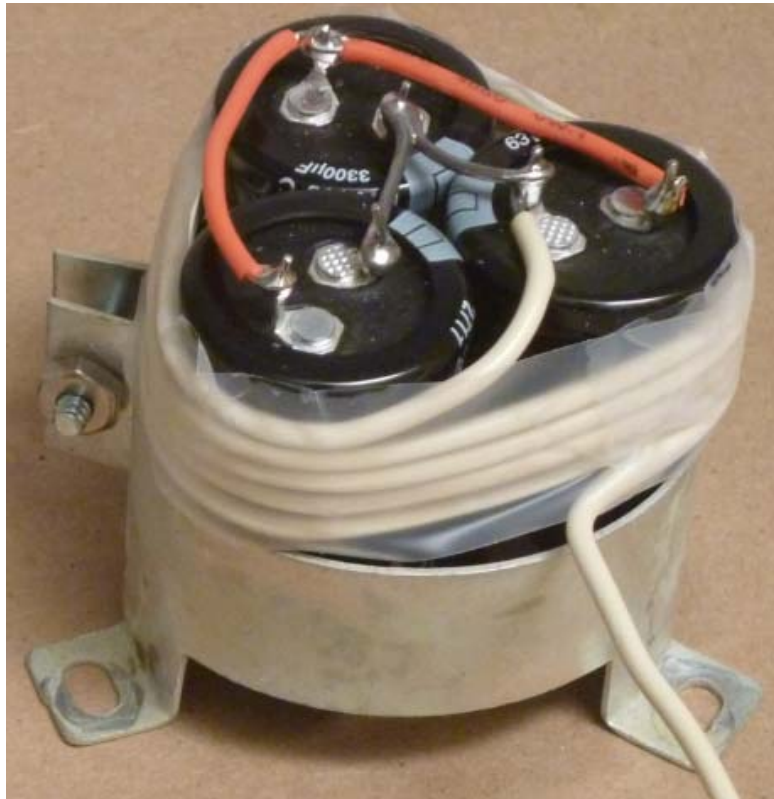
Figure 11-Adding red wires to connect positive terminals
