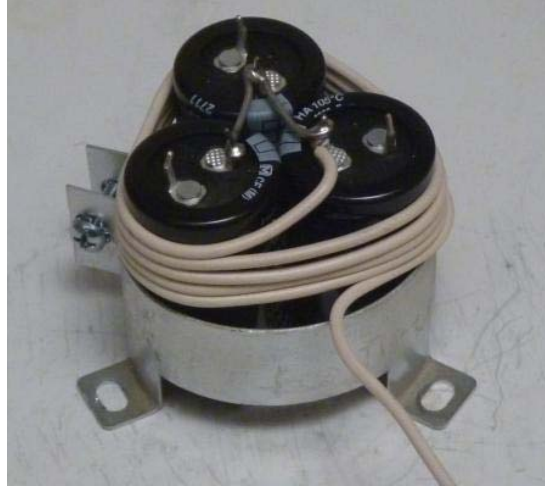
Figure 10-Inductor wound around the new C7
