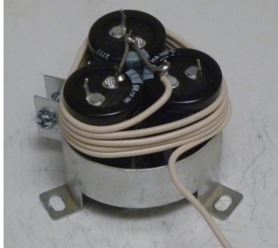
Figure 11-Inductor wound around the new C7
