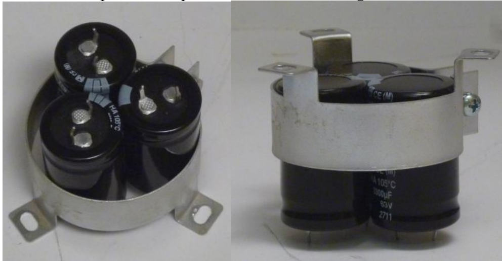
Figure 8-3 25 mm diameter capacitors take the space of one 2” diameter capacitor
