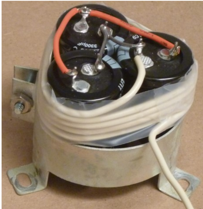
Figure 12-Adding red wires to connect positive terminals
